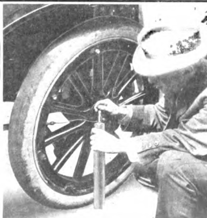
Fig. 4—Application of tube to tire
